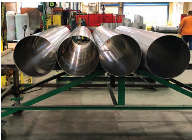
Efficient rolling of repetitive pieces such as alloy manifolds, 8' duct sections rolled to 14" OD.
