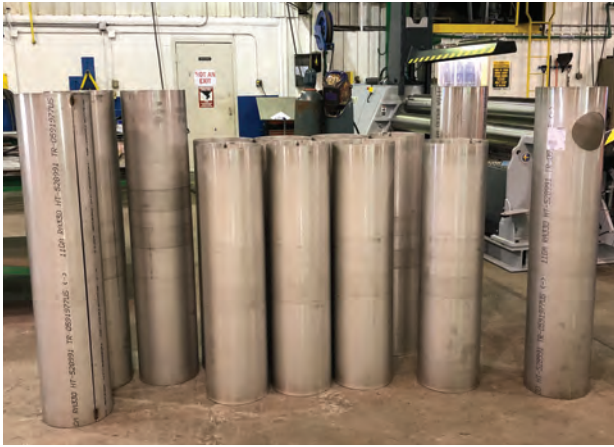
Dependable precision for high-grade material such as 330 alloy, 8' and 10' duct sections rolled to 14" OD.
