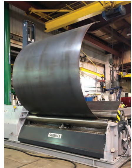
Rolling 3/8" Carbon steel 96" x 204" to 121" diameter.
