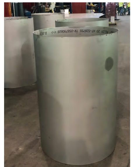
5' Alloy 20 duct sections rolled to 32" OD.
