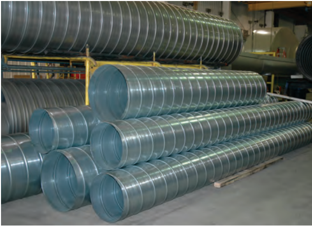
Spiral pipe available in 16–28 gauge, 3"–72" diameter.
