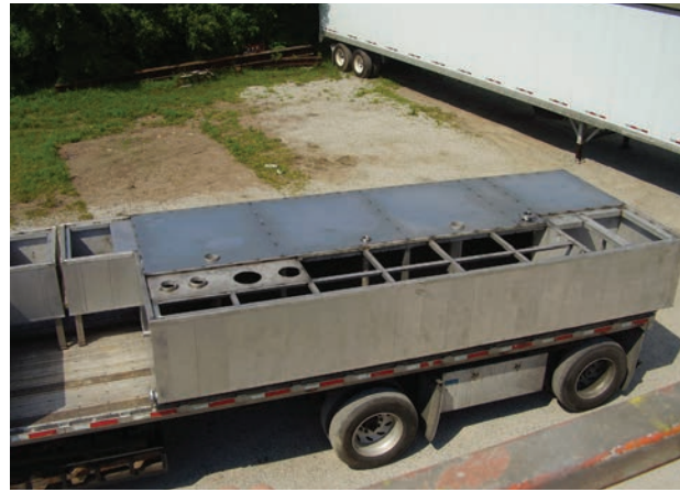
304 SS wash tank for appliance manufacturing customer.
