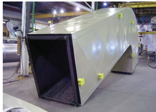
Carbon steel duct with shop-installed insulation & lagging.
