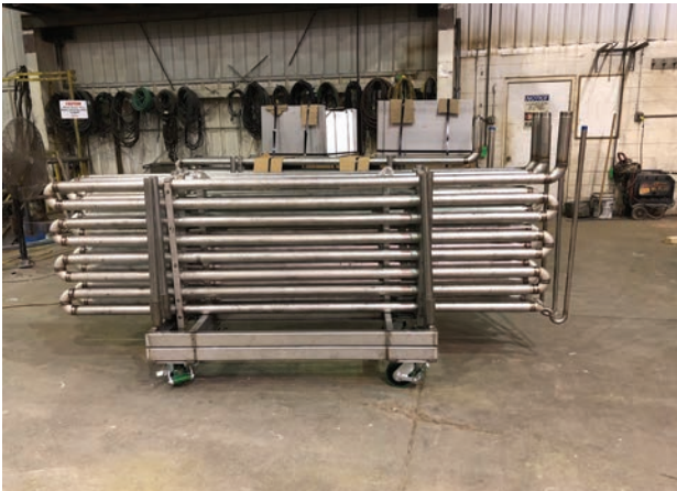
Stainless steel steam heat exchanger and mobile cart.
