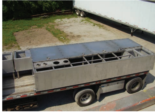
304 SS wash tank for appliance manufacturing customer.
