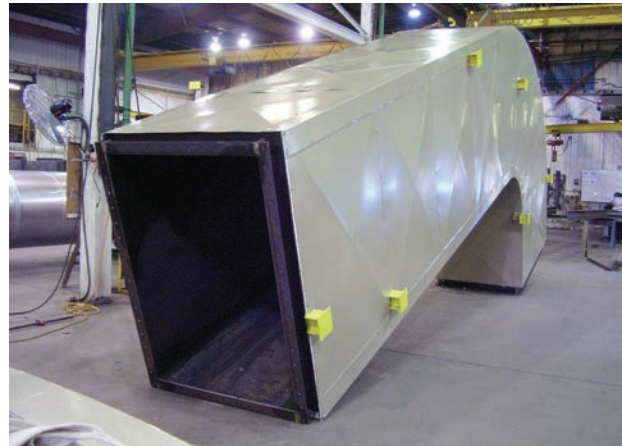
Carbon steel duct with shop-installed insulation & lagging.
