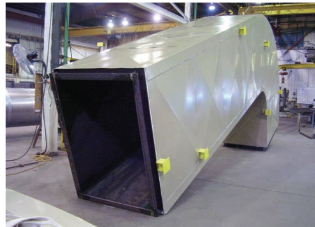
Carbon steel duct with shop-installed insulation & lagging.
