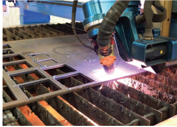
Beveling 1/2" carbon steel plates.
