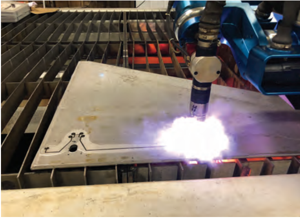
Plasma cutting 330 Alloy with air and water shielding for more precise cut.
