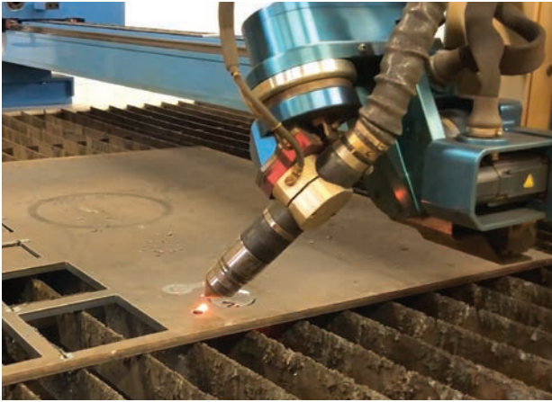
Plasma cutting countersunk hole in 1/2" carbon steel
