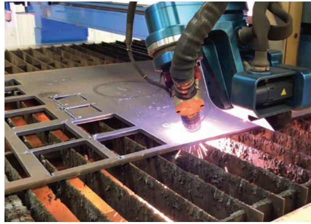
Beveling 1/2" carbon steel plates
