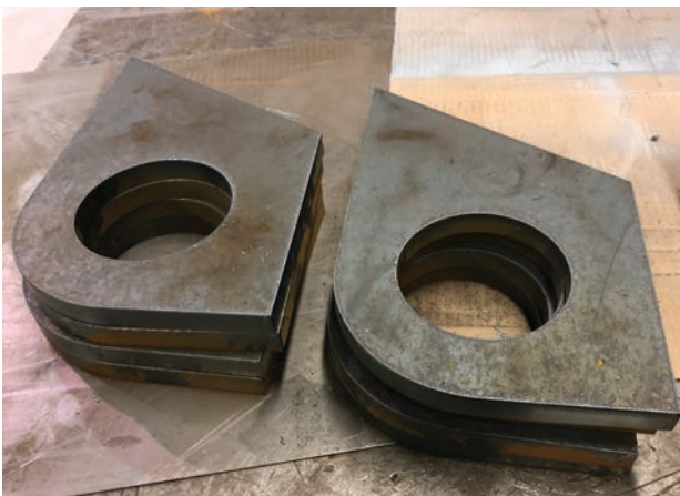
Plasma cut parts in 3/4" carbon steel
