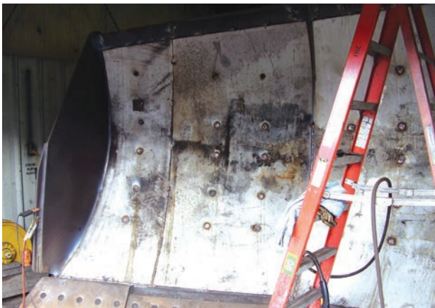
Repairing and reskinning energy customer's large dozer blade.
