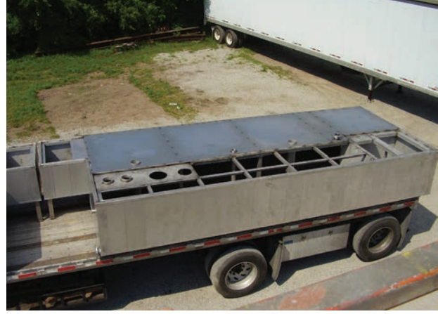
304 SS wash tank for appliance manufacturing customer.
