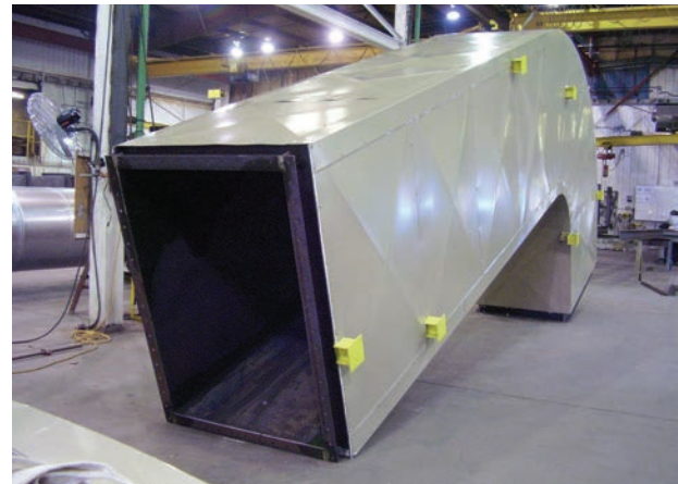
Carbon steel duct with shop-install installation & lagging.
